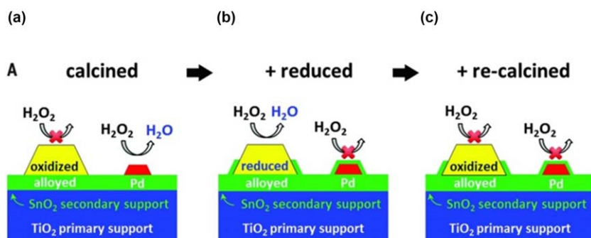
Scheme 8 Selective PdSn catalysts are created by (a) oxidation (calcined), forming a \text{SnO}_2 secondary support, then (b) reduction to cover the small Pd clusters with the \text{SnO}_2 so they cannot undergo secondary decomposition of \text{H}_2\text{O}_2 , and (c) a final oxidation step which suppresses the PdSn alloy from decomposing/hydrogenating \text{H}_2\text{O}_2 . Reproduced with permissions from S. J. Freakley, Q. He, J. H. Harrhy, L. Lu, D. A. Crole, D. J. Morgan, E. N. Ntainjua, J. K. Edwards, A. F. Carley, A. Y. Borisevich, C. J. Kiely and G. J. Hutchings, palladium-tin catalysts for the direct synthesis of \text{H}_2\text{O}_2 with high selectivity, Science , 2016, 351, 965. Copyright 2016 American Association for the Advancement of Science (AAAS).
